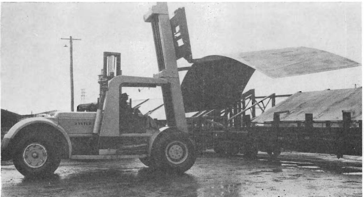
Unloading sheet steel with high capacity fork lift truck.
