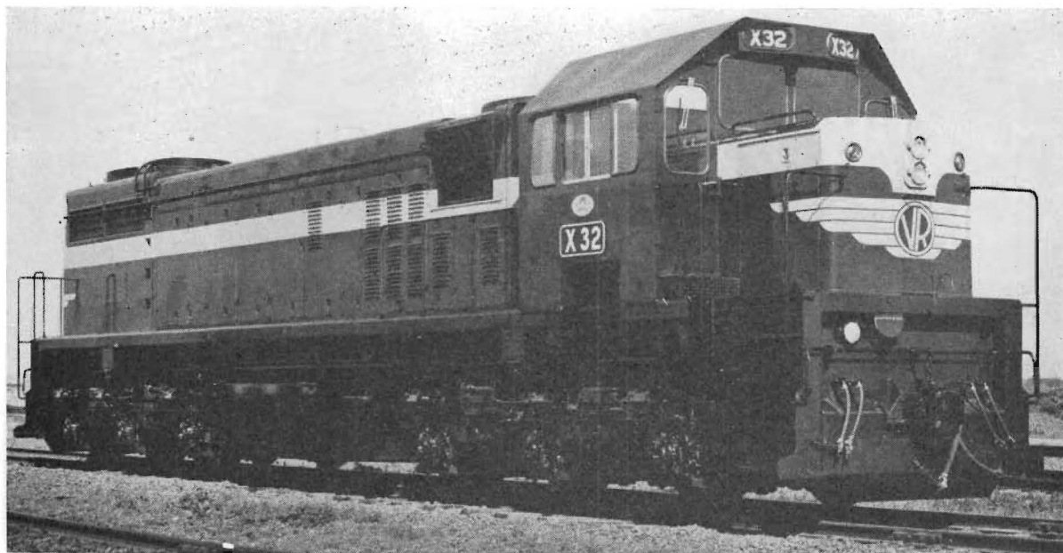
"X" Class 1,800 h.p. diesel-electric locomotive.
